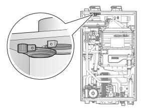
6. Remove the filter from the plastic assembly and clean it with a toothbrush and clean running water.
