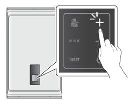
You can adjust the temperature while the display is flashing. Once the display stops flashing, the temperature setting is stored.
