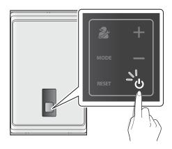
When the power is on, the boiler supply water temperature will appear with the water pressure on the front panel display in 5 second intervals.
