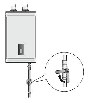
Close off any heating zones that do not require draining and open a purge valve to drain the space heating side. Open all domestic hot water faucets completely to drain the water heating side. The water that remains in the plumbing lines will drain out.
