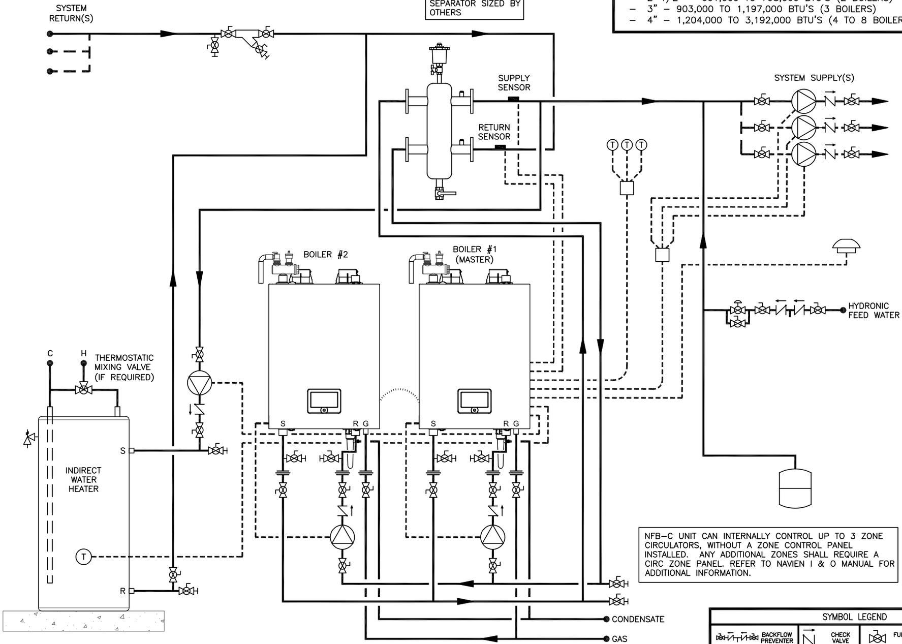
NFB-C UNIT CAN INTERNALLY CONTROL UP TO 3 ZONE CIRCULATORS, WITHOUT A ZONE CONTROL PANEL INSTALLED. ANY ADDITIONAL ZONES SHALL REQUIRE A CIRC ZONE PANEL. REFER TO NAVIEN I & O MANUAL FOR ADDITIONAL INFORMATION.
