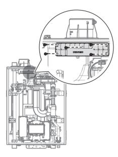
3. Remove the filter from the boiler and replace with a new filter.
