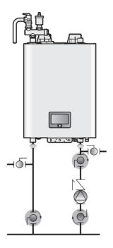
Remove the drain valve on the manifold system to drain the boiler.
