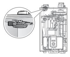
Remove the filter from the plastic assembly. Dust and rinse it with clean running water.
