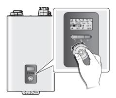
2. Press the Command dial ( ) to select the space heating temperature. The highlighted section will flash.
