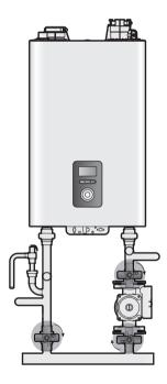
5. Remove the drain cap on the manifold system to drain the boiler.
